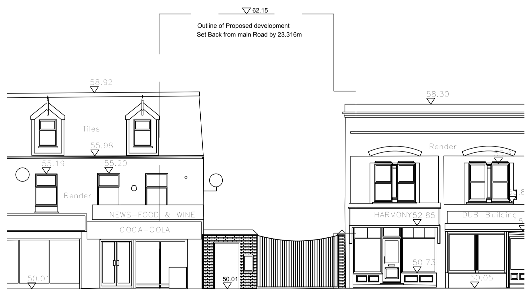
02 PROPOSED South Street elevation REF. 14175 SCALE: 1:100 (A1)
